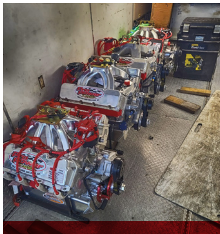
Bill Schlieper provided this photo of the kinds of engines Pro Power Racing brings for track support (left to right): a 450 D3 Ford, Chevy 10-degree wide-bore 440 package, Chevy 11-degree 454 wide-bore, and a 436 Ford RY45 package.
