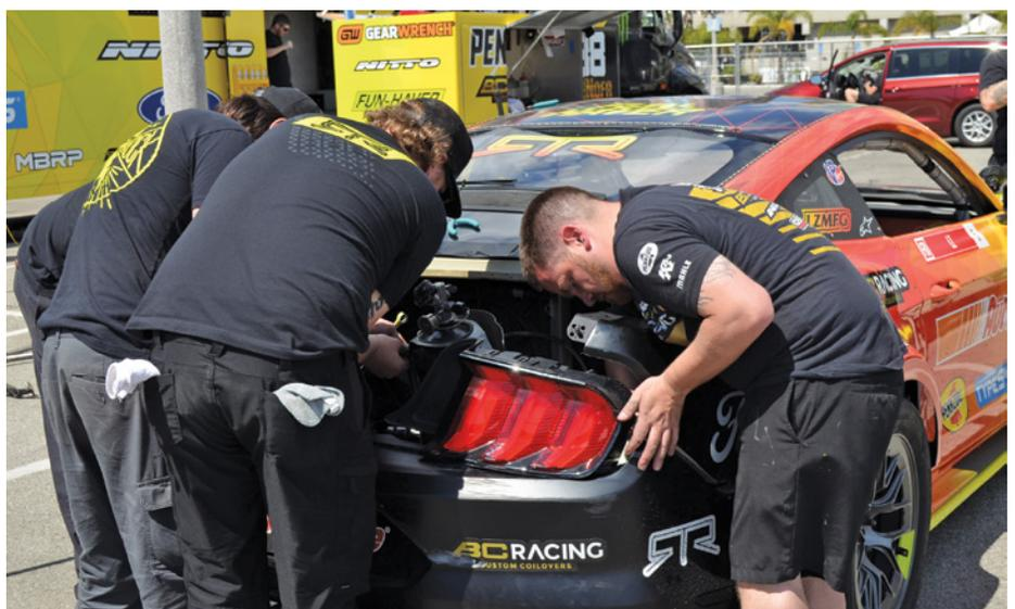
Because contact is not uncommon in drifting, most teams bring spare aftermarket bumper structures and other body components to make them easier to replace between heats, "especially for the rear," said Kevin Wells of Formula Drift.
