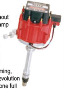
To advance or retard the timing, simply turn the knob (1/2 revolution equals 1 degree of timing; one full revolution equals 2 degrees of timing).
