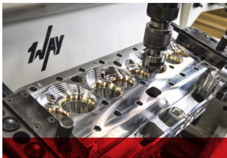
Creating a clean-sheet cylinder head can require months of development work. 1 Way Technologies discovered new efficiencies when it came up with a way to produce GM SB2 and ROX cylinder heads from a single casting.
