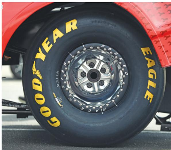
The friction stir welding process Race Star Wheels uses for its Pro Forged line results in a wheel that's "lighter and stronger, which really helps 60-foot times because the wheel is more true than a wheel that's been welded together in sections," said Race Star's Brian Sexton. "Even in Funny Car, with Cruz Pedregon [seen here], the cars just come off the line and don't shake the tires."
