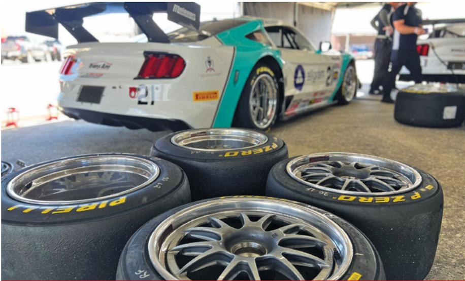
Forgeline supplies competitors ranging from SCCA club racers to the elite of IMSA and WEC road racing. All of its wheels are forged and are designed for load rating “and sometimes aero,” said David Schardt. “Aero puts an extra load on the wheel; 1,000 pounds of downforce is like putting an extra 1,000 pounds on the car.”
