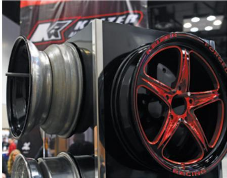
Keizer Aluminum Wheels are cold-spun using aerospace quality aluminum "to meet precise tolerances," said Wade Huisman. "Our forged billet blanks are CNC machined in-house" at the company's Iowa facility. The wheels are manufactured for customers driving anything from Pro Street to formula cars.
